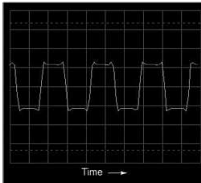
Figure 7.31: Oscilloscope time-domain display of a square wave
